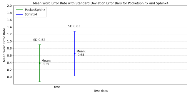
Figure 11: Mean Word Error Rate for Sphinx4 and Pocketsphinx for the NCHLT test data
