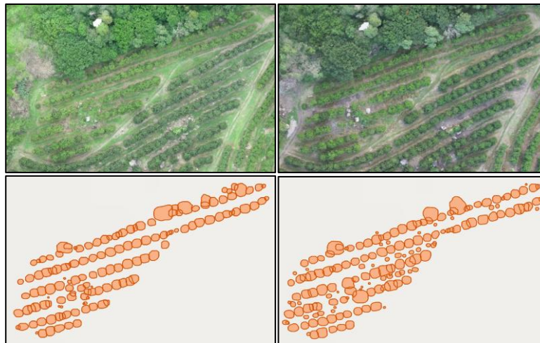
Figure 1: Multi-temporal orthomosaic maps of an orchard (top) and their corresponding feature detections (bottom).
