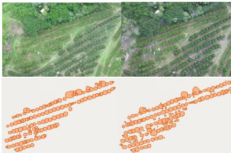
Figure 1: Multi-temporal orthomosaic maps of an orchard (Top) and their corresponding feature detections (Bottom).
