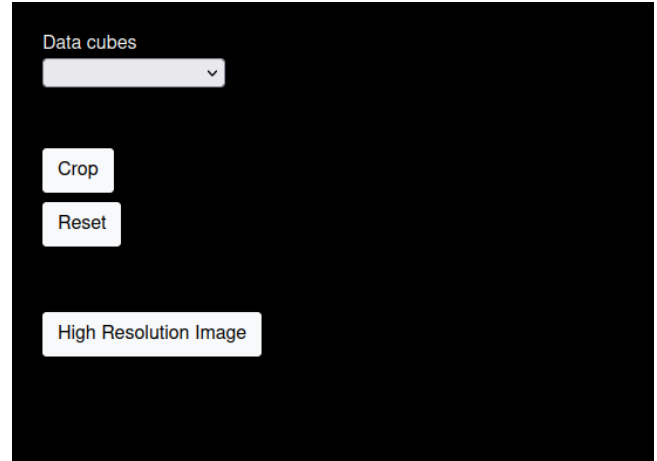
Figure 4: The user interface of the client system before the user has selected a file with a drop down selection element to allow the user to view and select a file as well as the the other function the user can perform on the data cube, such as crop the data cube, reset the page and request a high resolution image if desired. The rest of the screen is blank.
