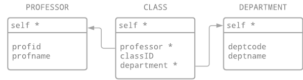
Fig. 1. ARM schema showing a simplified university system
