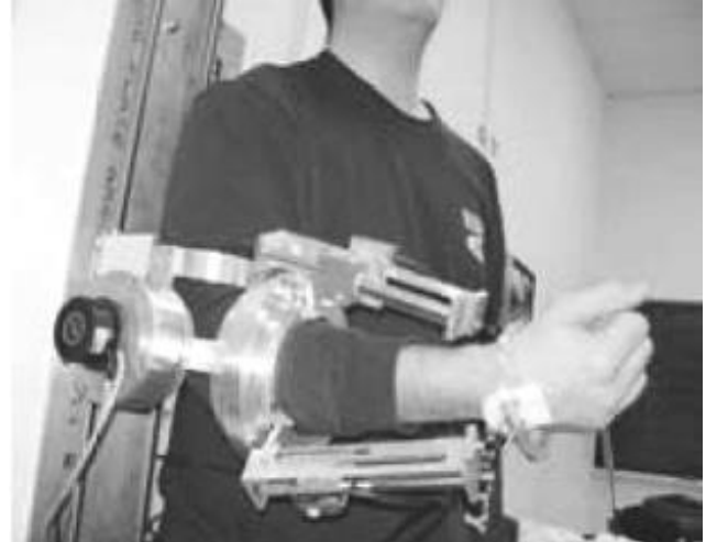
Figure 1 - User operating the exoskeleton [Gupta and O'Malley 2006]
